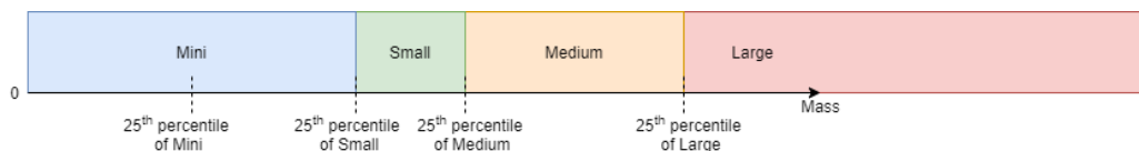
Figure 4: A diagram demonstrating how missing segments are imputed by matching a vehicle's average mass to the 25th percentile of known segments' mass.
